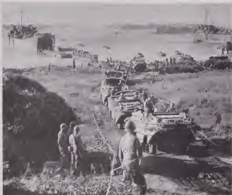
FIGURE 21. DUKWs landing at Anzio. The beach exit, specially paved with landing mat sections, is rarely required by DUKW unless beach is muddy.
